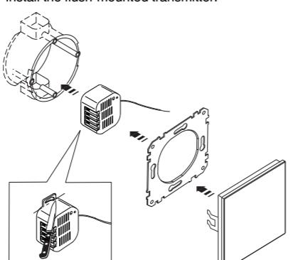
**i** Place the antenna as far as possible from metal parts (connecting cables, retaining rings, etc.) to avoid interruptions to the radio signal.
