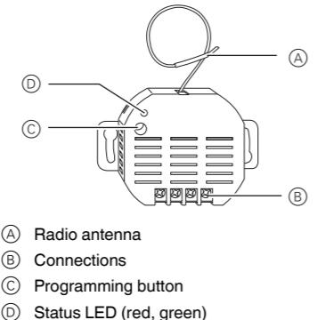
**Installing the flush-mounted transmitter****DANGER****Risk of death from electric shock!**
