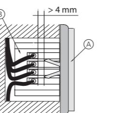
If the distance is less than 4 mm, you must use either a deeper installation box or a different cover! The fixing brackets or screws of the cover must not press against the housing.
