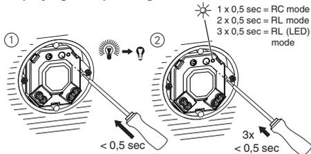
The circuit breaker is switched on. **(Live working!)**
