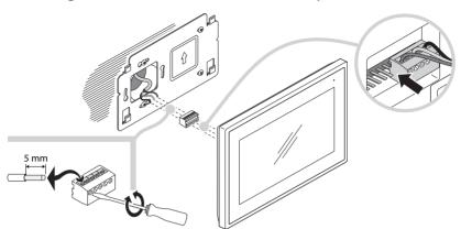
1 Perform connection according to the wiring diagram.
