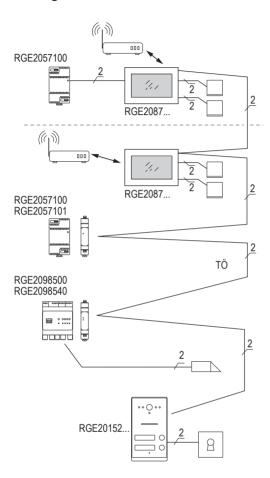
For information on connecting the indoor station with a router see Block diagram --> 15 in chapter Single-family house.
