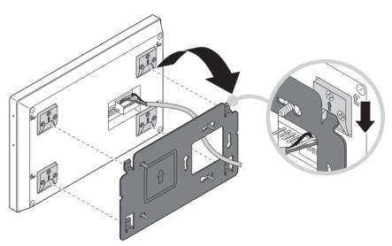
② Insert the indoor station on the base plate.
